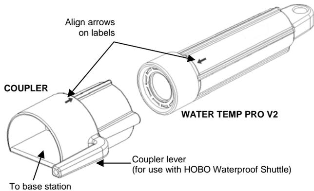
5. If you are using the HOBO Waterproof Shuttle, briefly press the coupler lever to put the shuttle into base station mode.
