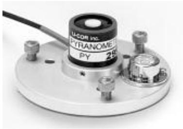
Figure 2: LI200S pyranometer
