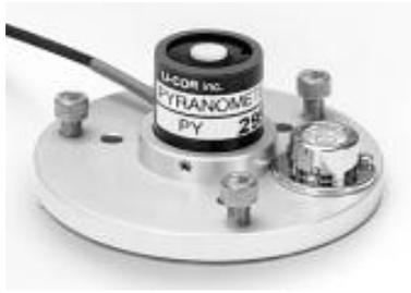
Figure 2: LI200S pyranometer
