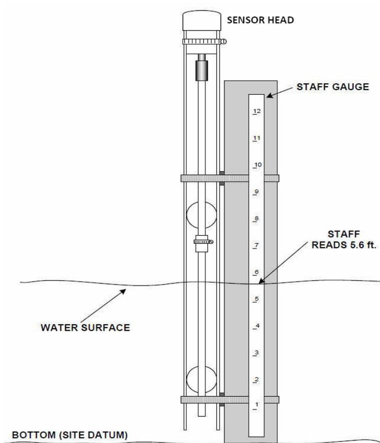
Figure 9: Aquatrak Tide Gauge Installation
