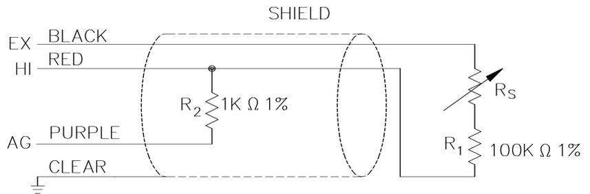
FIGURE 1. 237 Sensor Schematic
