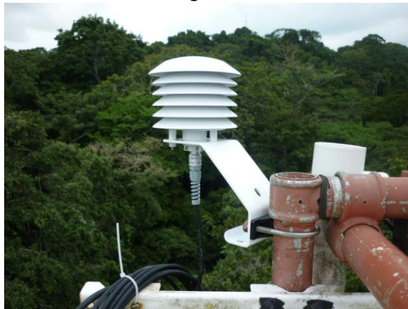
CS215 sensor Temperature & Humidity sensor inside 6-gill naturally aspirated radiation shield
