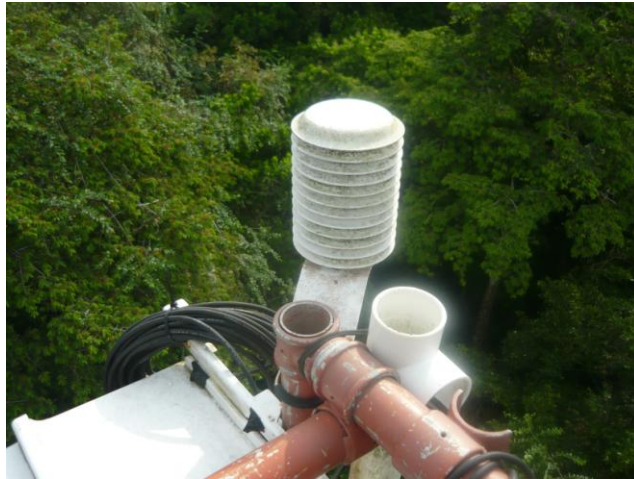
HMP 45C sensor Temperature & Humidity sensor inside 10-gill naturally aspirated radiation shield
